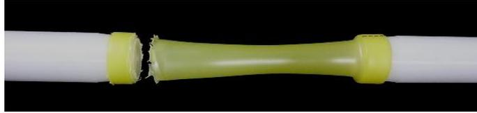
Fig.6 Appearance of broken tension test specimen
