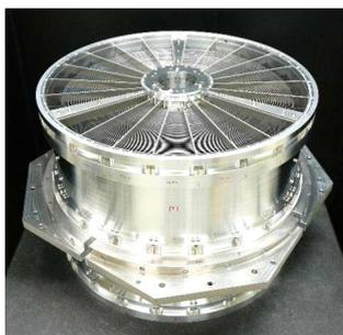
Fig. 11 Schematic of assembled HXT reflector.
