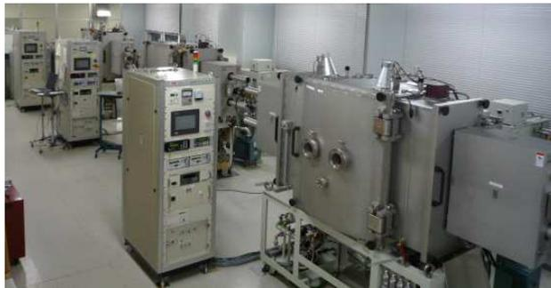
Fig. 7 DC sputtering system used for HXTs (Nagoya University).
