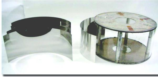
Fig. 8 Photographs of glass-pipe mandrel (right) and HXT reflector (Pt/C multilayer supermirror) released from mandrel (left).
