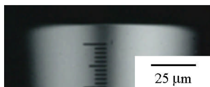
(b-1) Flank face (before machining)
