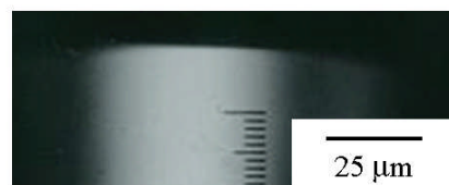
(b-2) Flank face (after machining)
