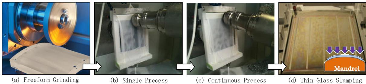
图 5 Process chain #2 for fabricating aspheric hard X-ray shells
