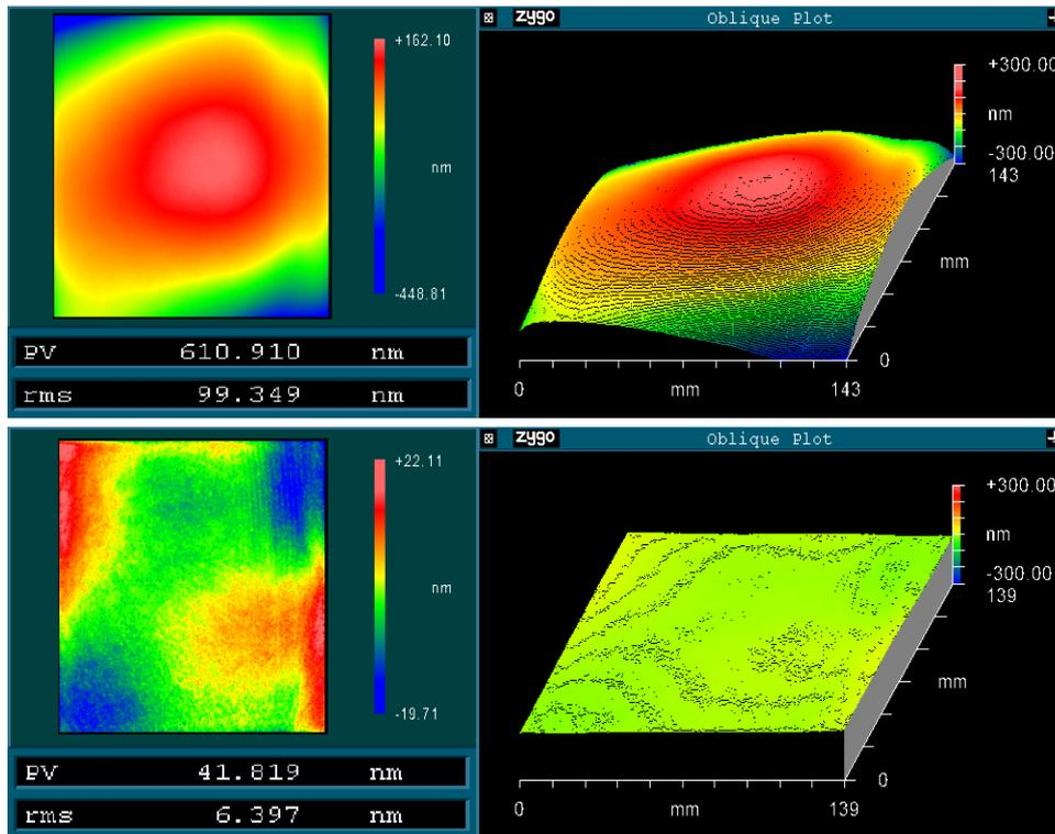
图 7 Form Correction on Fused Silica by Precessed Bonnet Polishing
