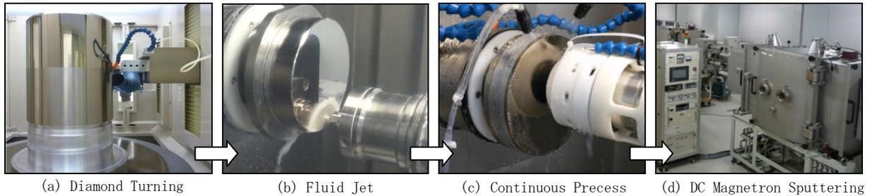
图 4 Process chain #1 for fabricating aspheric hard X-ray shells
