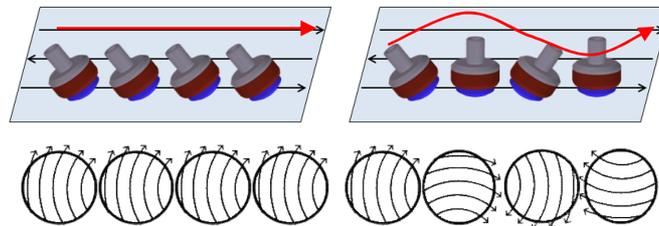
图 10 Single (left) and Continuous Precessing (right) across Raster Tool Path.
