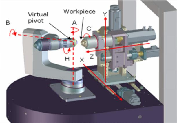
图 3 7-axis CNC platform used for fluid jet and bonnet polishing.
