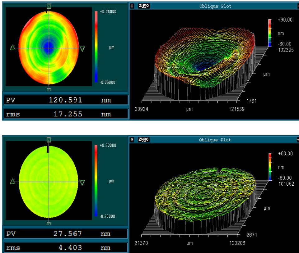
☒ 6 Form Correction on Electroless Nickel by Fluid Jet Polishing
