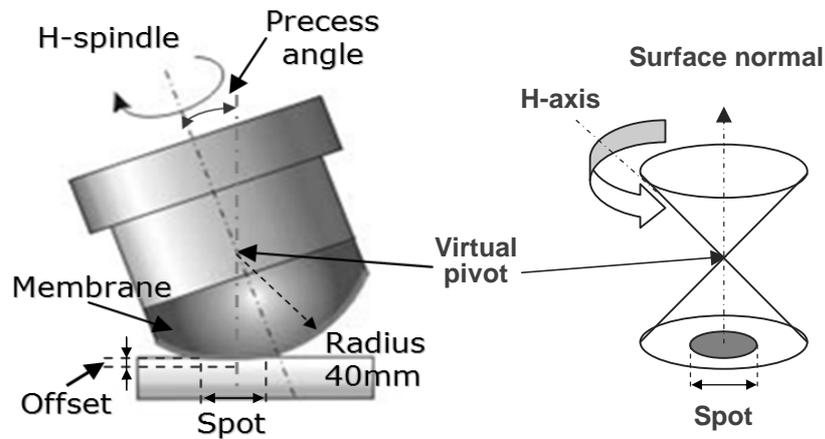
图 9 Precessed Bonnet (left) and “Continuous Precessing” (right).
