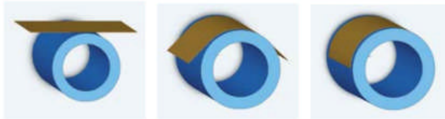
图2 Slumping thin glass over Wolter Type-1 mandrel
